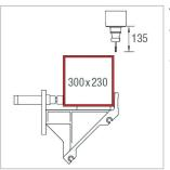
Traverse path, Y and Zaxes SBZ122/74 Profile machining from
